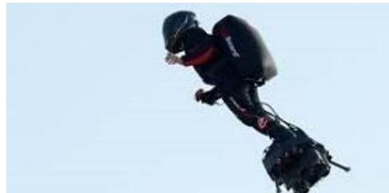
Zapata invented the Flyboard in 2011, a device that uses a water jet to propel the rider through the air behind a boat. He later invented the Flyboard Air, a board powered by four turbo jet engines that allows a rider to fly through the air untethered, using a computer to keep it stabilized.
