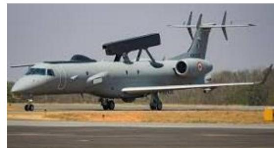
Netra is useful for surveillance, tracking, identification and classification of airborne and sea surface targets and is useful in detecting incoming ballistic missile threats.
