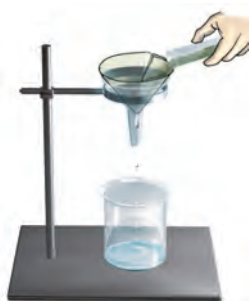
Fig. 5.10 Filtration using a filter paper
