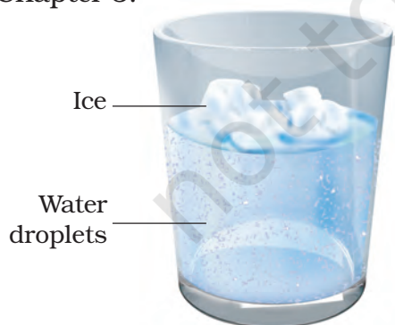
Fig. 14.6 Drops of water appear on outer surface of the glass containing water with ice
