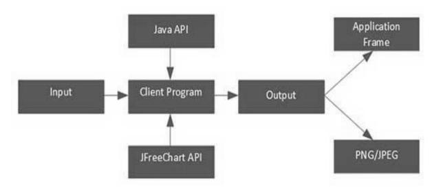
The client program receives user data and then it uses standard Java and JFreeChart APIs based on requirements to generate the output in the form of either a frame, which can be displayed directly inside the application or independently in the image formats such as JPEG or PNG.
