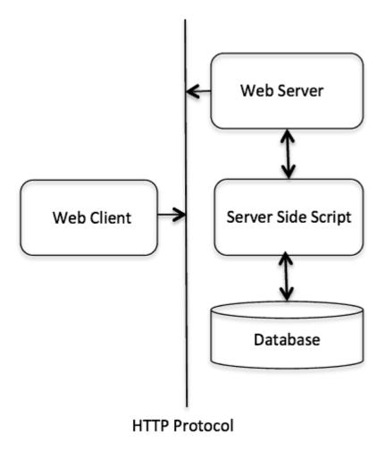
The HTTP protocol is a request/response protocol based on the client/server based architecture where web browsers, robots and search engines, etc. act like HTTP clients, and the Web server acts as a server.
